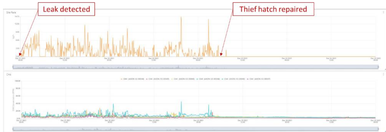
Figure 12 - Site rate and methane concentration detecting an open thief hatch during Enhance's Alt-FEMP with Qube's CM system
